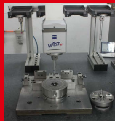
ZEISS三坐标测量仪检测 3A-110004零点卡盘 ZEISS coordinate measuring machine detects Zero Point Chuck 3A-110004
