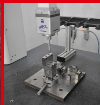
ZEISS三坐标测量仪检测 3A-200002旋转摆动式虎钳 ZEISS coordinate measuring machine detects Rotatable Pendulum Vise 3A-200002
