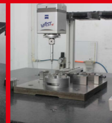
ZEISS三坐标测量仪检测 ITS卡盘 ZEISS coordinate measuring machine detects ITS Chuck
